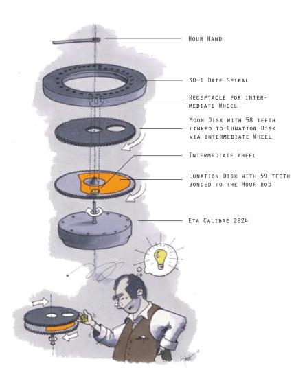
Ludwig Oechslin has managed to create this indication using just four components. True to his credo *the simpler, the better*, the mechanics that underlie the indication are easily understood.
